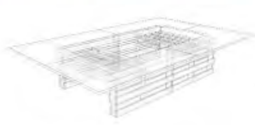
The Conference Table. The conference table is primarily made from wooden pallets and reuse table platforms as its surface.
