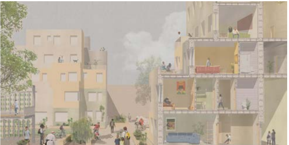
Mohsin Ali - Sectional perspective of the western housing block showing the relationship between the hempcrete-timber structure, units, interior street circulation, farm and landscaping
