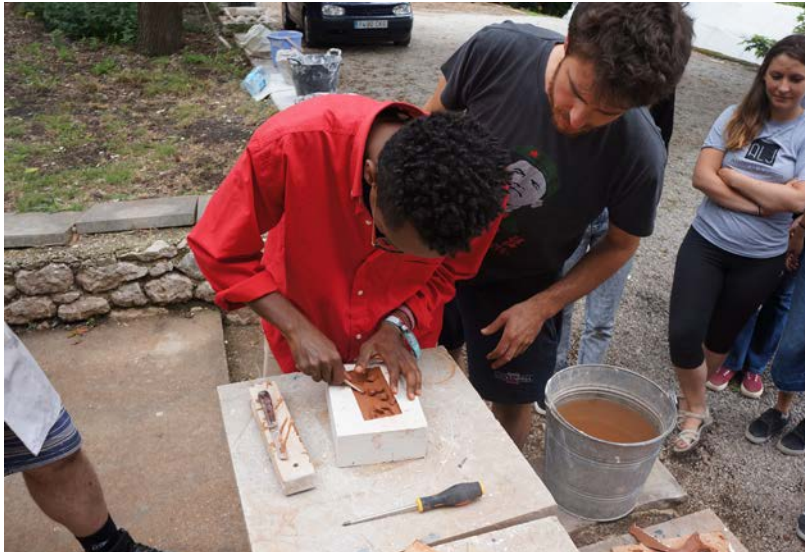
Atelier La Juntana, Summer School - preparing a plaster mould for clay tile production
