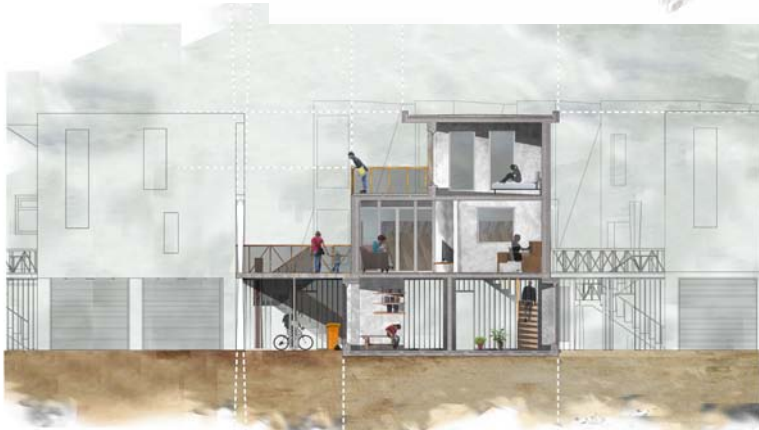
The section of the 2 storey house demonstrates the different levels of the dwelling. The 2 garages underneath, offer create an independent space from the main upstairs living area. The raised living spaces create a section that only residents can use therefore adding a level of privacy and security at that level.
