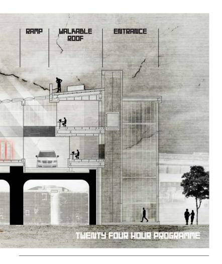
The walkable roof structure allows people to disembark from the station and circulate over the building. Views down into the data centre, through the ETFE roof ensures the presence of the data can always be tangible throughout the journey through the scheme.
